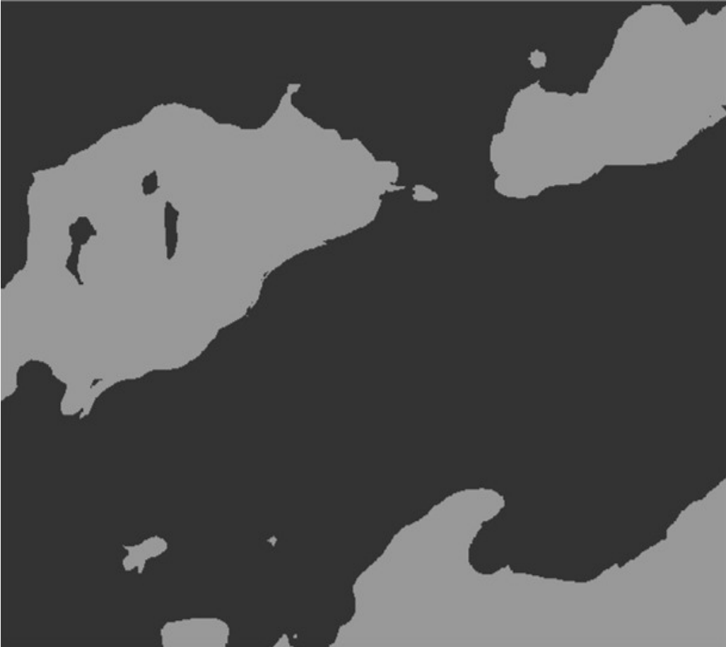
Figure 8. Layered and clustered zones derived from elevations and EM readings, Mansfield. This image was derived using a combination of ArcMap to register the elevation and EM maps, then were imported into ERDAS Imagine as a .img file. The files were layered, and the layers were subjected to unsupervised classification using the isodata clustering method embedded within Imagine. This map shows the higher landscape positions being segregated from the rest of the field.
